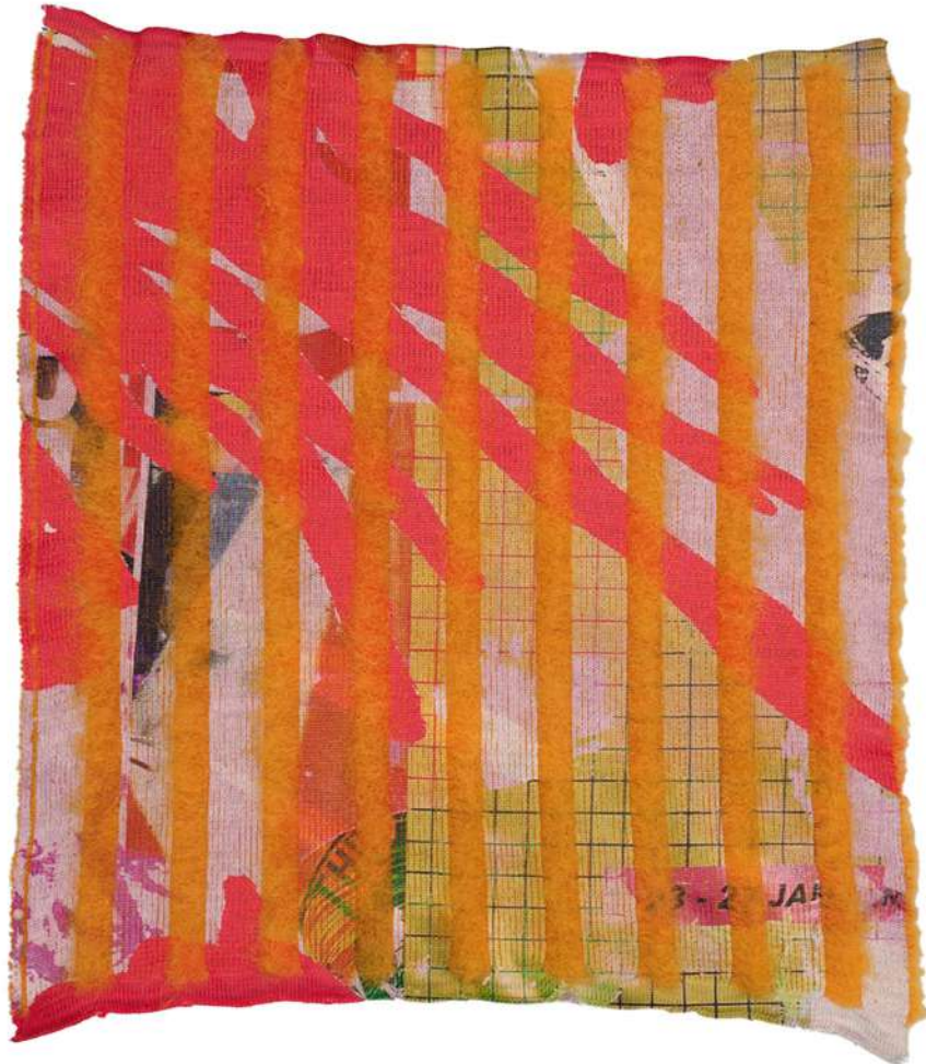
MOHAIR INLAY AND SUBLIMATION PRINT 10X10 INLAY SET UP ON 10 GAUGE INDUSTRIAL MACHINE SUBLIMATION DYE BY HEAT PRESS
