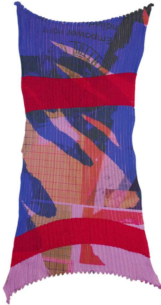
SUBLIMATION PRINT ONTO RIB 4X2 RIB SETUP ON 10 GAUGE INDUSTRIAL MACHINE
