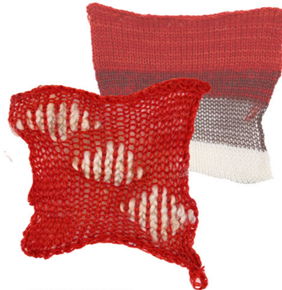
-Chunky domestic machine -Tension 1 -Ewrapping sheeps fleecing - Wool
