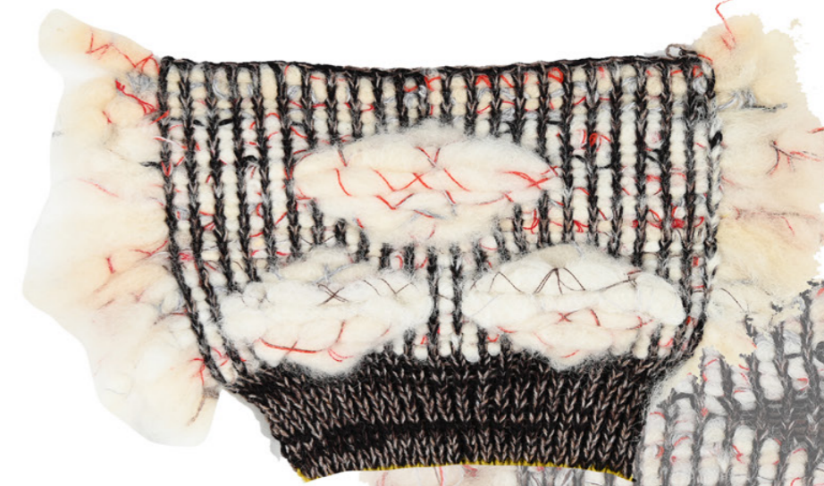
-Dubied Industrial machine -Gauge 3 -Tension 20 -Inlaying sheeps fleecing - Wool
