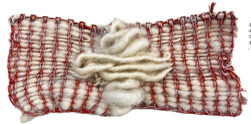
-Dubied Industrial machine -Gauge 3 -Tension 22 -Inlaying sheeps fleecing - Wool
