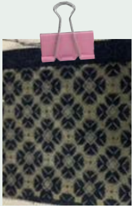
This pattern was created through repeating an image of lace to create a print. The print then got raster engraved onto denim.
