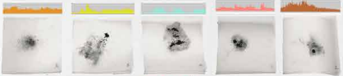
Observe the diffusion of pencil dust by placing it on a stereo and playing different tones of music at different frequencies.
