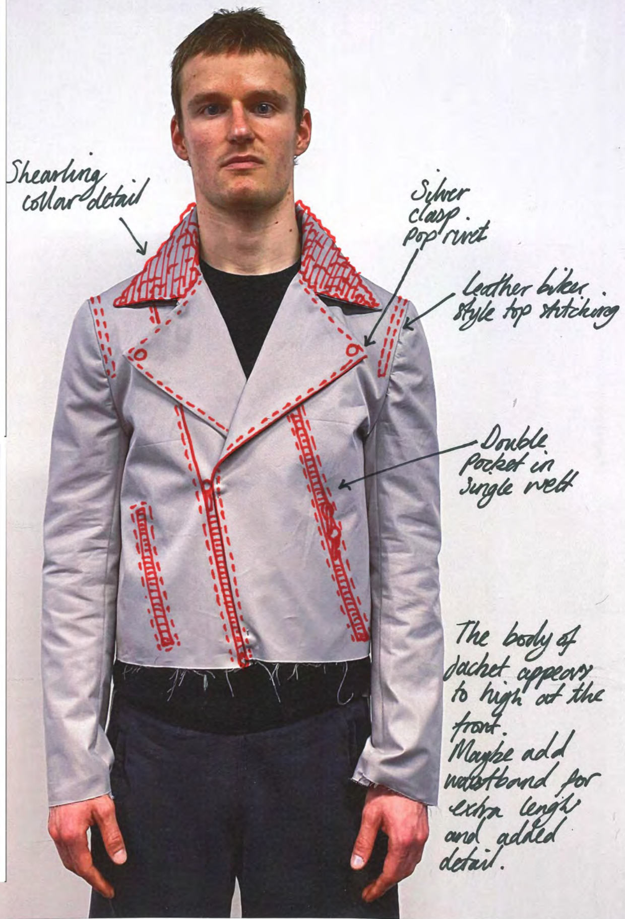
Initial biker jacket est - toile in grey cotton twill. Missing waistband and shearling collar detail. Zipper welt pockets to be marked.
